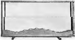
FIG. 1.—Vertical Section of Mound raised from Level Sand by Oscillating Water.
